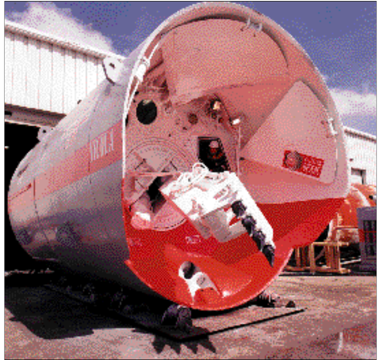
Photo 4.3.3 - Compressed air TBM - Boom type
