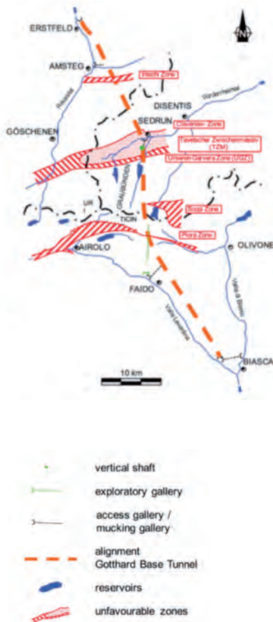
Figure 15 : Alignment of the Gotthard Base Tunnel (Switzerland) in relation to unfavourable ground conditions
