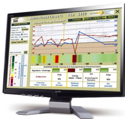
Figure-11: BEAM INTEGRAL user interface 2012; e.g. simultaneously indication of BEAM forecast results on a monitor placed outside the tunnel; BEAM results indicate a cavity zone of about 2m thickness and medium water content in a distance of about 4m ahead of the face yet, whereby the first detection was shown 20 m ahead of the face
