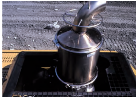
Figure 20 : Use of particle filters is part of the concept for environmental protection (© AlpTransit Gotthard Ltd)
