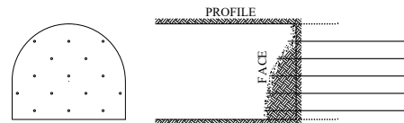
g. Pre-excavation Injection (Prel)
