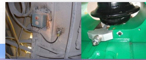
A0 (+) measuring electrode (e.g. cutter head, excavation tools)
