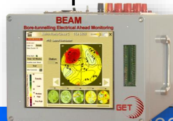
BEAM unit (placed in operator cabin)
