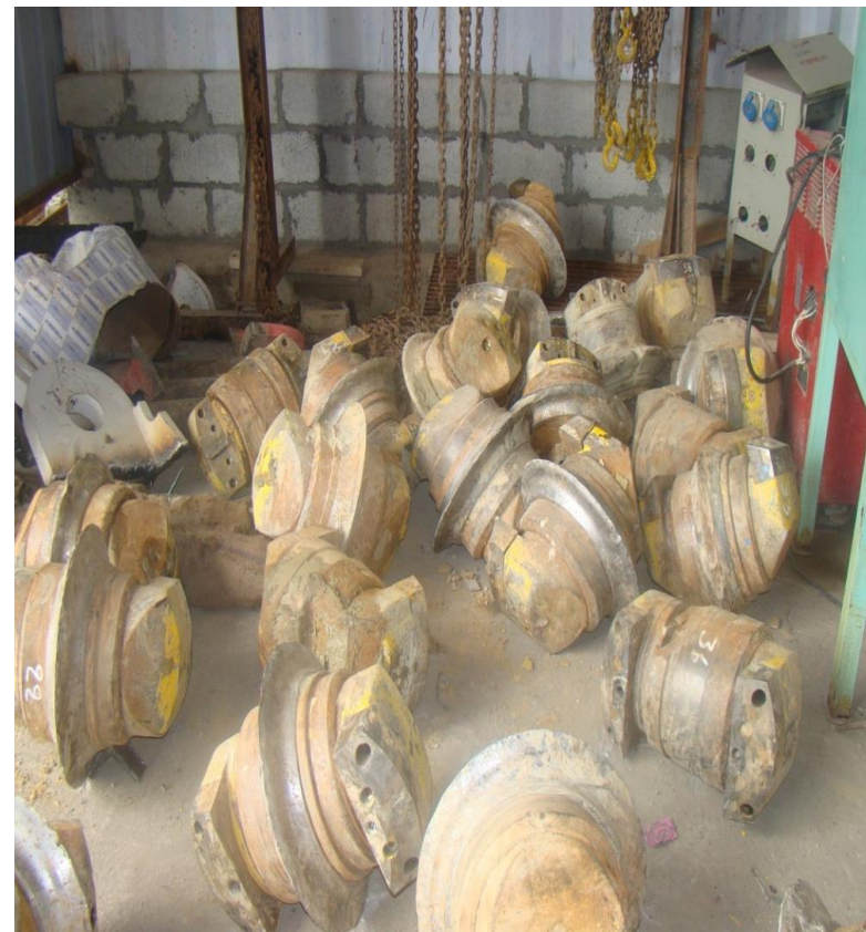
DAMAGED CUTTER DISC
