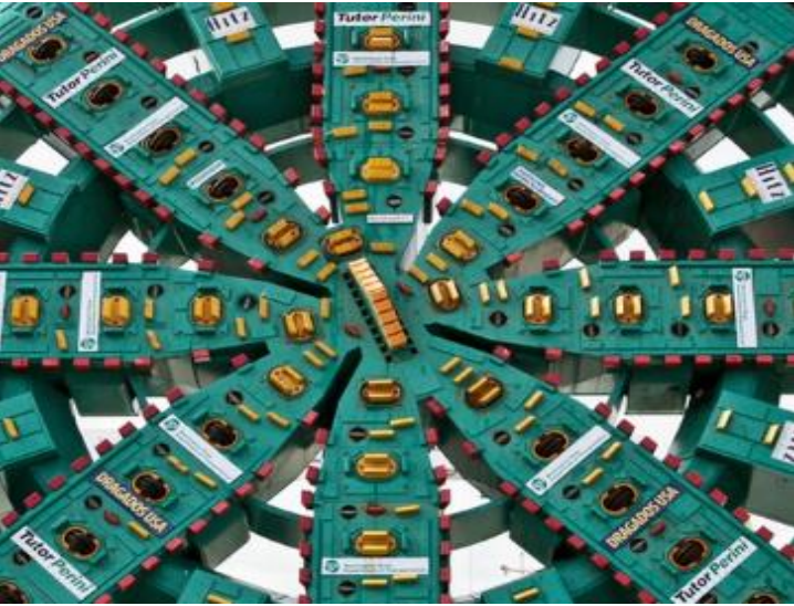
EPB TBM for Soft Grounds
