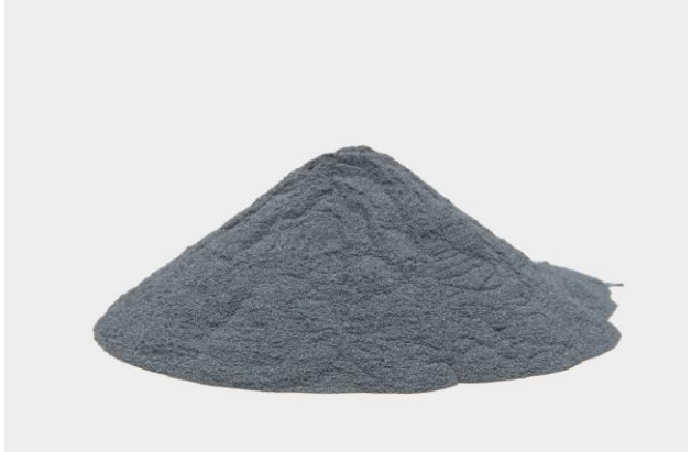
Silica fume is 100 times finer than cement
