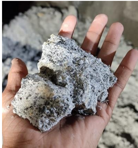
Crushed Dolomite mixed with PU-2C grout
