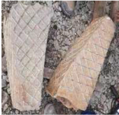
Fig. (5a) Broken mixing arm
