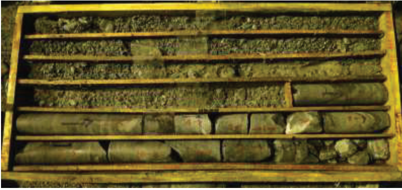
Fig 11: Hard rock found at chainage 2454 by core drilling
