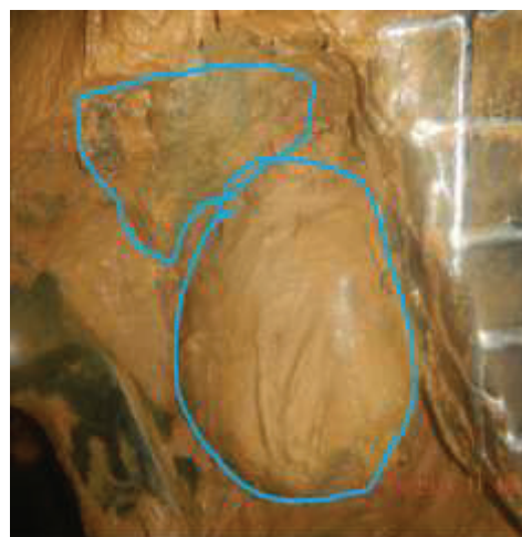
Fig. (7b) Boulders between cutting tools
