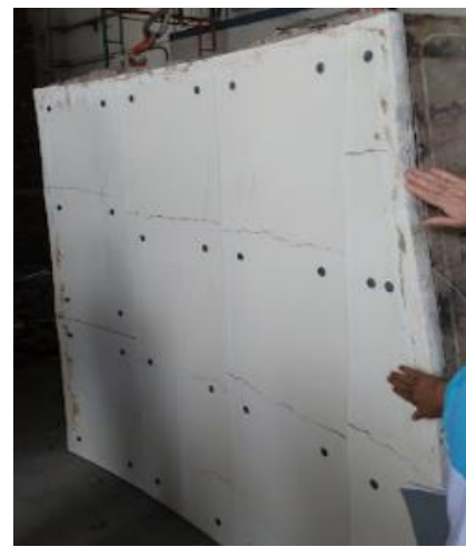
(b) Fire Board Samples after the Test
